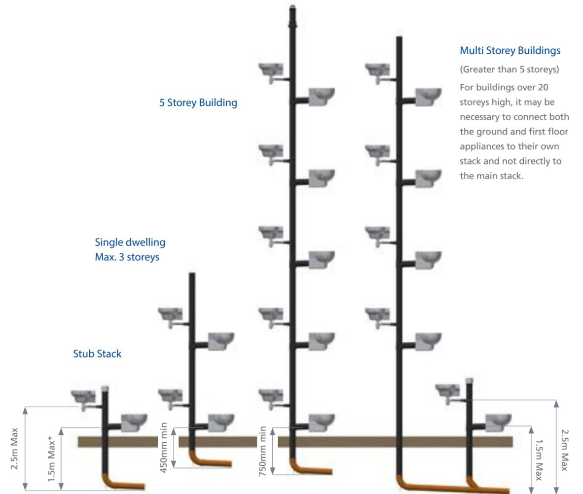
\* BS EN 12056-2 states 1.5m from the invert of the pipe to the centre line of the branch.
