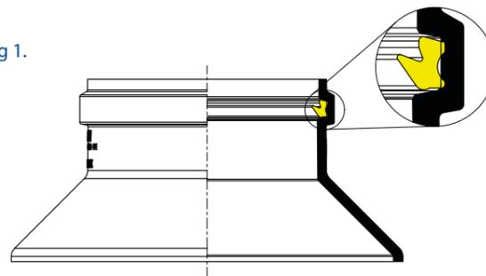
NOTE: On low pitched roofs, optimum weathering may be achieved by making a single weld to the lower edge of the base plate.
