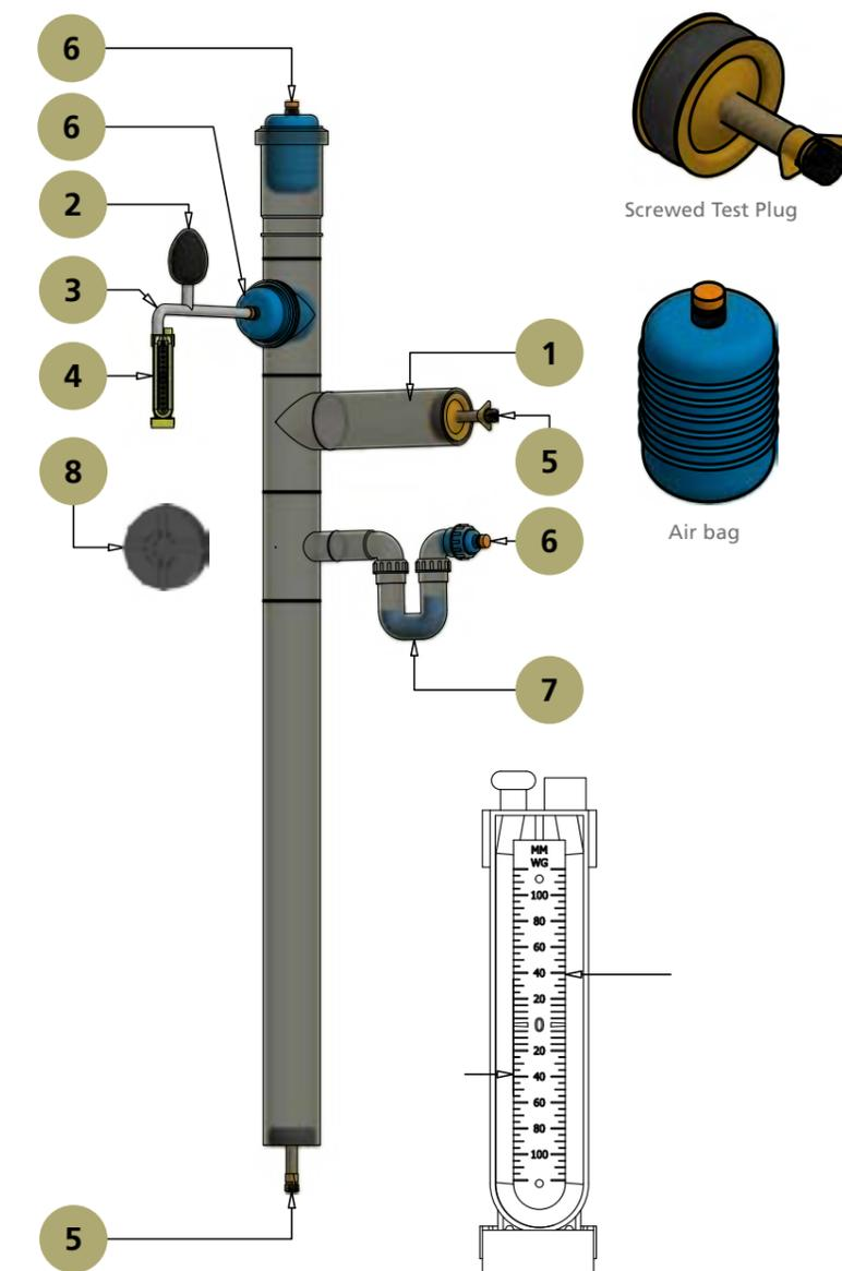
**Note:** Blue temporary caps are not to be used for air pressure testing, only black threaded caps are to be used. Further information is available on technical bulletin:2016 - PT06 - Air pressure test to comply with BS EN 12056-2 - Version 6
