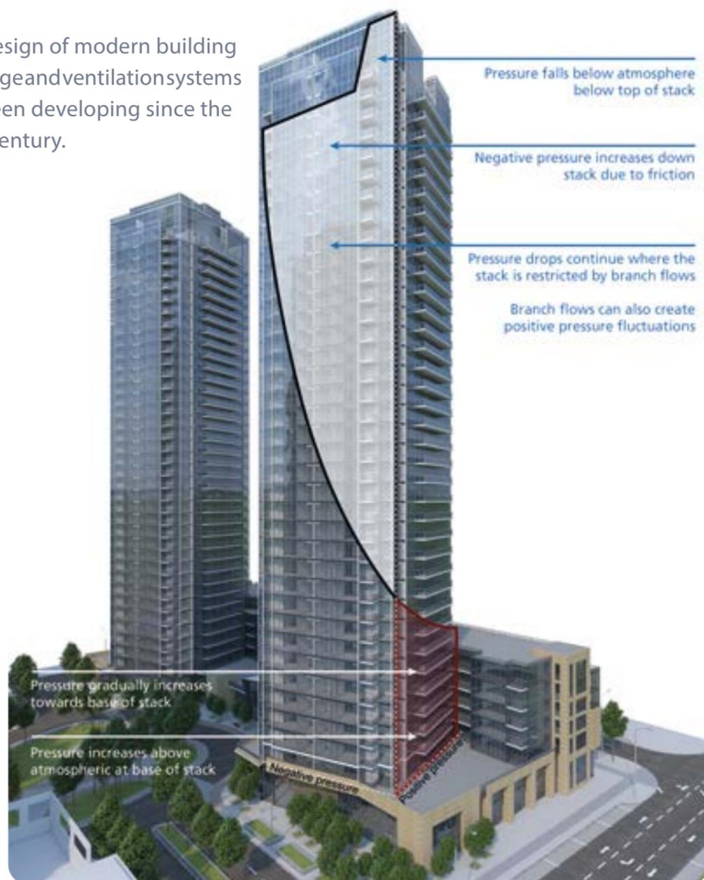
A minimum of 50mm of water is all that protects the occupants of a building from potentially harmful sewer gases and 'particulates'. Therefore, a good design must consider the integrity of the trap seal and protect it from being lost. One way of doing this is to consider the air flow within the system, as this is the primary reason for trap seal breach. The flow of air within the drainage pipework system is equally as important as the flow of water in maintaining a safe and
