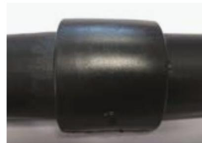
In the joint to the right the pipe has not been cut square and you can also see that the pipe surface has not been scraped. This joint is likely to leak.
