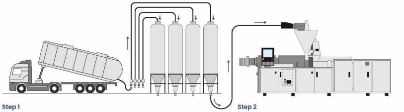
Raw material is delivered to our factory on a tanker and deposited into our silos.
