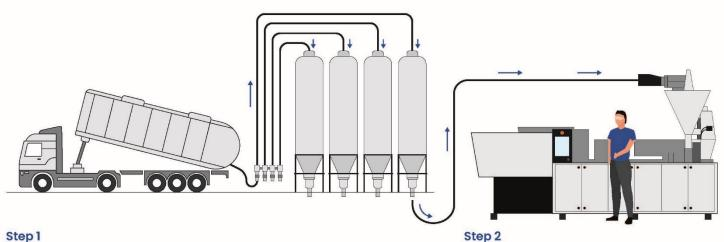
Raw material is delivered to our factory on a tanker and deposited into our silos.
