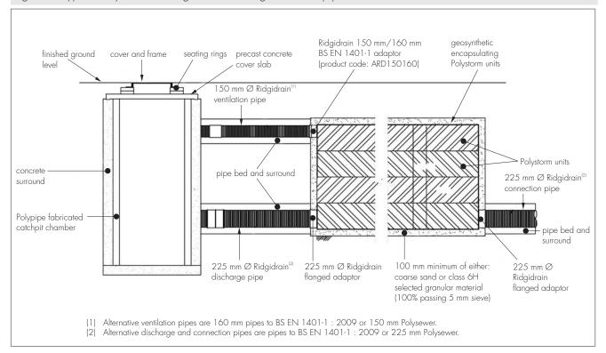
Figure 4 Typical Polystorm-R arrangement including ventilation pipe
