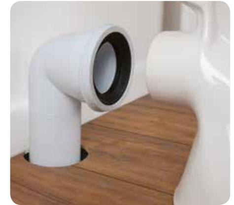
3. Once the pan connector is inserted into the pipe the toilet can be positioned and installed to the pan connector. When the toilet is in position it can be fixed in place.
