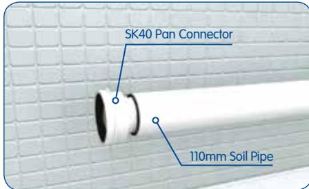
Pan connectors are manufactured from polypropylene and all versions have a 110mm spigot outlet for connection to a ring seal soil system socket. This type of connector is not suitable for solvent welding.
