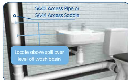
appliances are connected to the soil stack, the access point should be sited above the spillover level of the appliances.
