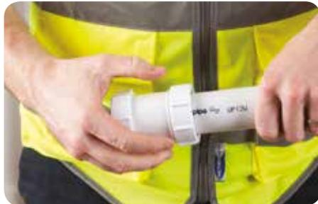
6. Screw the threaded nut onto the body of the fitting. Once tight apply an additional 1/4 turn.
