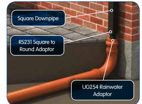
*Downpipe discharging into Universal Drain Adaptor*
