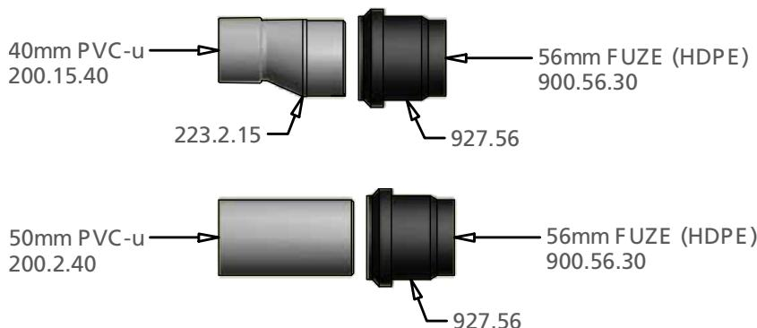
The only two waste sizes which are the same between PVC and HDPE are 50mm PVC and 56mm Terrain FUZE, both 56mm outside diameter. This has meant that it is common practice for drainage stacks to be installed with a 56mm branch for easy adaption onto any PVC waste size with the use of level invert reducers.
