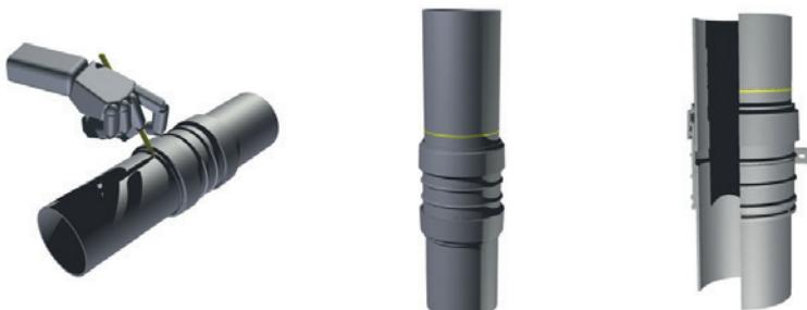
The pipe connecting into the ring seal adaptor should be inserted fully into the socket and marked. To create the expansion gap withdraw the pipe 12mm from the socket. This gap will allow the pipe to expand sufficiently without distorting the pipework.
