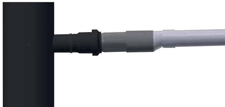
Adapting from one material to another can sometimes require a number of different fittings. An example shown (Fig. 1) shows a solution of bringing 32mm PVC waste into a 40mm Terrain FUZE HDPE branch. As you can see there is a requirement for a number of fittings to make this adaption.
